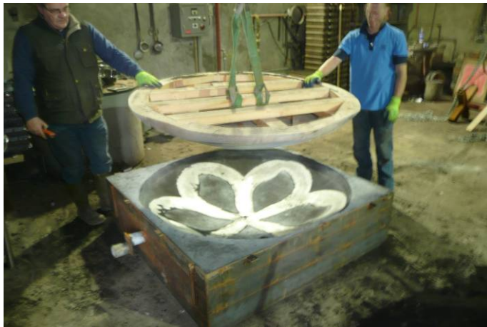
One petal component being cast
