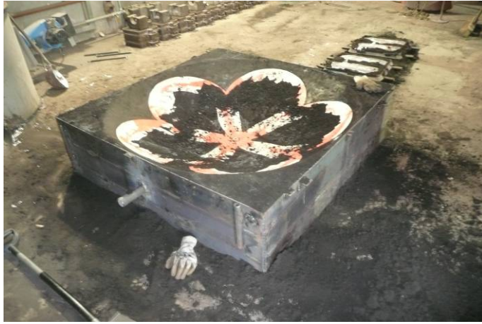
One petal component being cast
